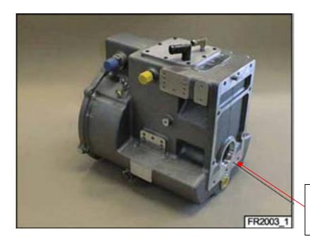
Gearbox/housing mating plane: LOCTITE 518 sealing compound
